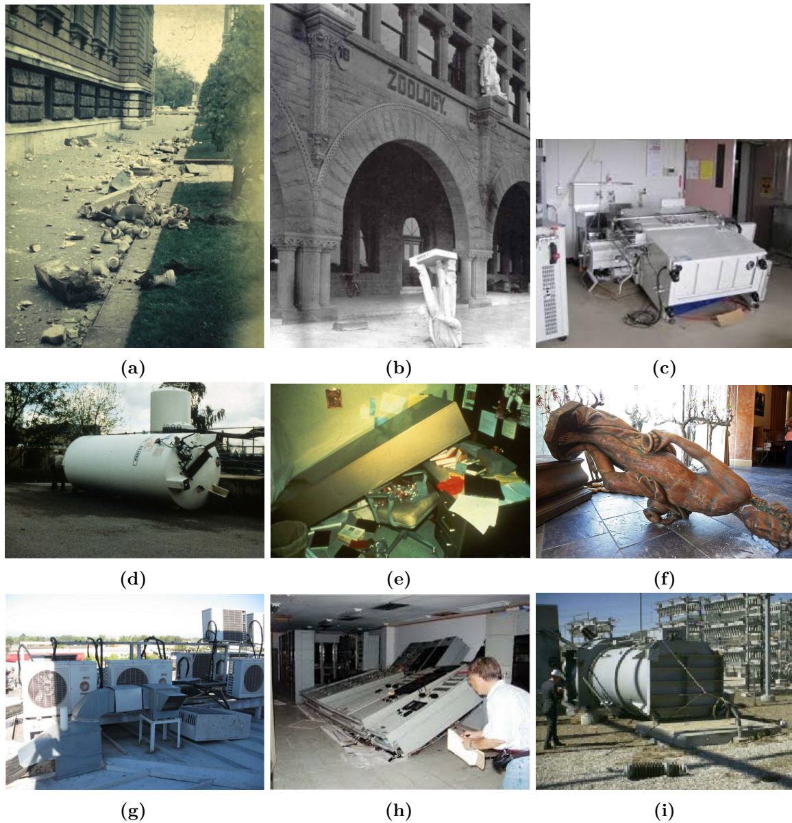
Fig. 1.2: Examples of earthquake damage to freestanding structures: (a) fallen balustrade on Vienna University-1972 Seebenstein earthquake (Photo/Walter Eppensteiner) [8], (b) the Agassiz statue-Stanford's 1906 earthquake (Photo/Frank Davey) [9], (c) overturned lab workstation-2011 Japan Earthquake [10], (d) toppled vertical tank, 1994 Northridge earthquake (Photo/OSHPD) [11], (e) overturned bookcase onto desk-1971 San Fernando earthquake [11], (f) overturned Statue fo Bachuss, a Roman god of wine inside the Ceja Vineyards tasting room-2014 South Napa earthquake (Photo/Reuters) [12], (g) roof top units-2010 Chile earthquake [11], (h) overturned equipment-1985 Mexico earthquake [11], (i) toppled electrical equipment-1971 Sylmar earthquake [13]
