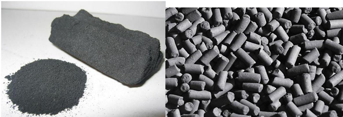
Abbildung 22: Links: Aktivkohle in Pulver- und Blockform
