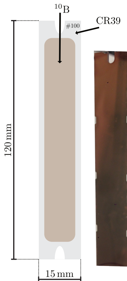
Figure 8.1.: On the left: CR39, 10 B detector dimensions. On the right: Photo of a CR39 plate detector with 10 B coating.
