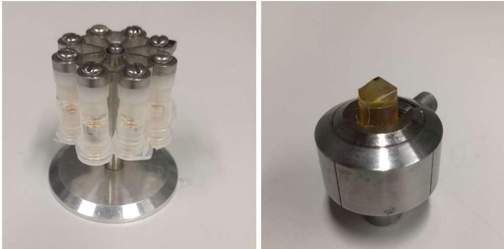
Figure 15 Polymerized HM20 samples on the unique spider web, which assists with the polymerisation, as the UV light is able reach the sample from all the sides, including the bottom. On the right: epoxy resin embedded trimmed sample.
