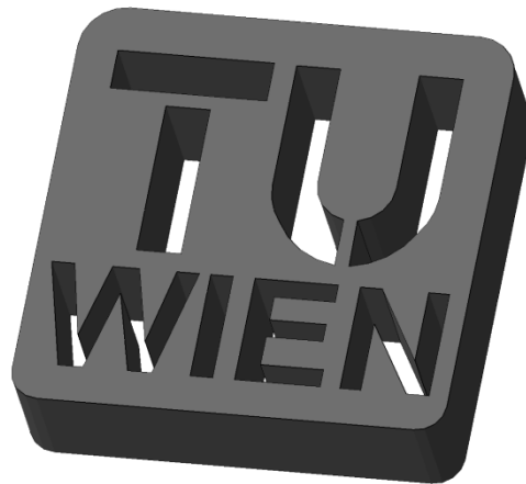
Figure 80: CAD-model of the TU Wien logo (dimensions 500 × 500 × 125 μm). The "top" layer in the picture is joined to a glass substrate, while the "bottom" is a through-polymerized lid (omitted in the picture for better visibility), so that the void "letter" areas are closed from all sides and allow trapping of cells.
