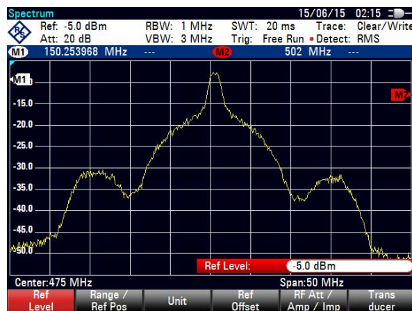
Figure 5.5: GPS L1 signal spectrum observed in the Experiment 179a and visualized with a spectrum analyzer connected to an intermediate frequency (IF) channel in Hobart. The depicted IF spectra is down-converted from the RF domain using a local oscillator frequency of 1100 MHz.
