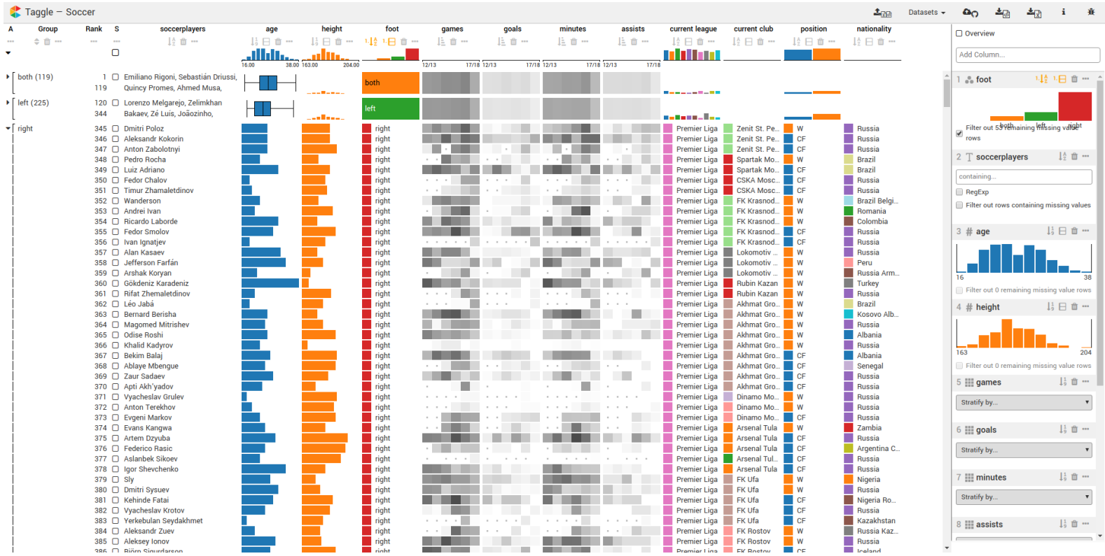
Figure 2.9: Taggle [25] with football player data in detail mode. While players who shot with either the left or both feet are aggregated, data for those who shoot with the right foot is displayed in detail. A box plot visualizes the aggregated items for the attribute age , and a histogram summarizes the aggregated items of attribute height .
