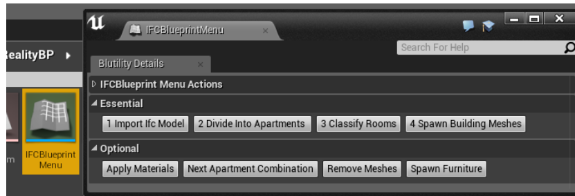
Figure 3.3: User interface of Unreal Editor — interactive blueprint that allows to (re-)trigger different steps of the processing workflow
