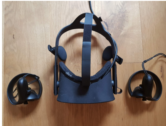
Figure 2.3: Head-mounted display Oculus Rift and its motion controllers Oculus Touch.
