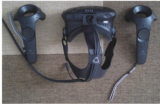
Figure 2.4: Head-mounted display HTC Vive with motion controllers
