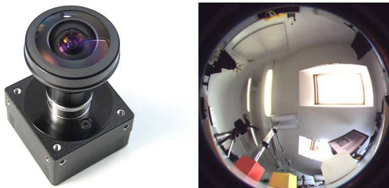
Figure 3.3: Left: Camera with a fish-eye lens used for real-time environment map capturing. Right: The image captured by this camera.
