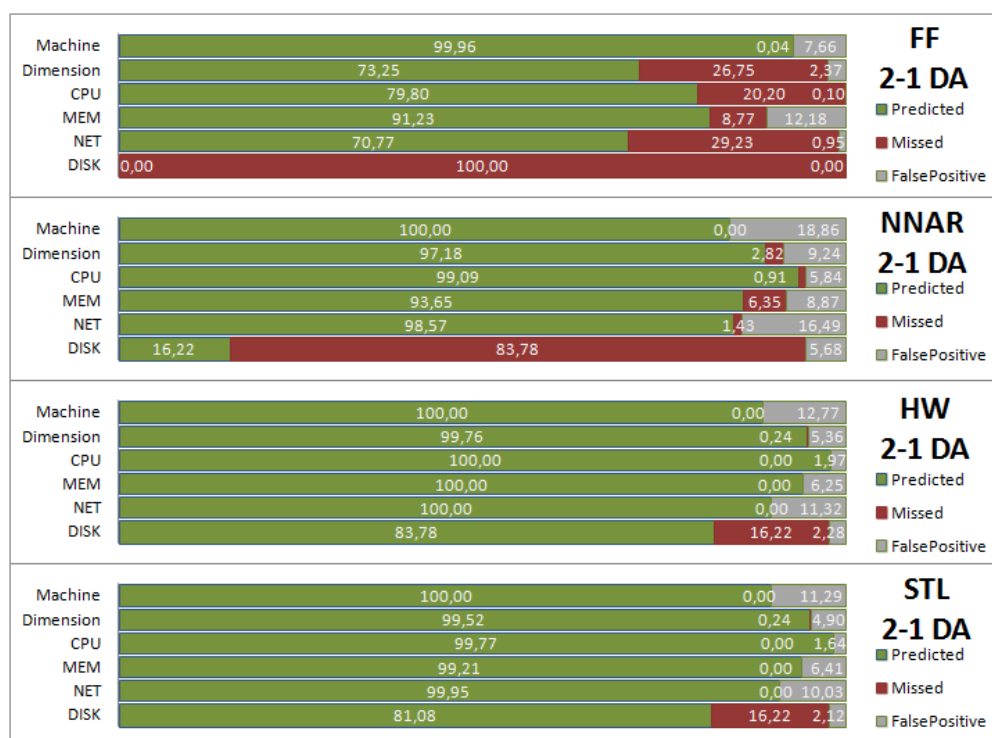
Figure 7.18: Results on 2days - 1 day split with dynamic error correction. Confidence level is set to 90% and window size is 30 data points. FF: Fourier forecast; NNAR: Neural Network AutoRegression; STL: STL (Seasonal and Trend decomposition using Loess) based forecasting; HW: Holt Winter's exponential smoothing; DSHW: Double Seasonal Holt Winter's exponential smoothing
