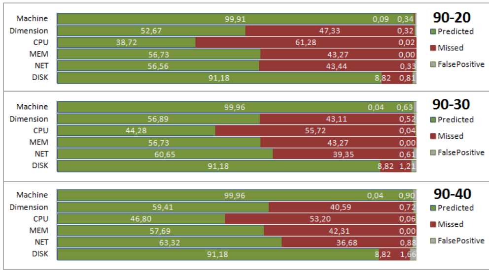
Figure C.4: STL forecast with changing confidence level. The first number in the chart title is the confidence level, the second is the window size.
