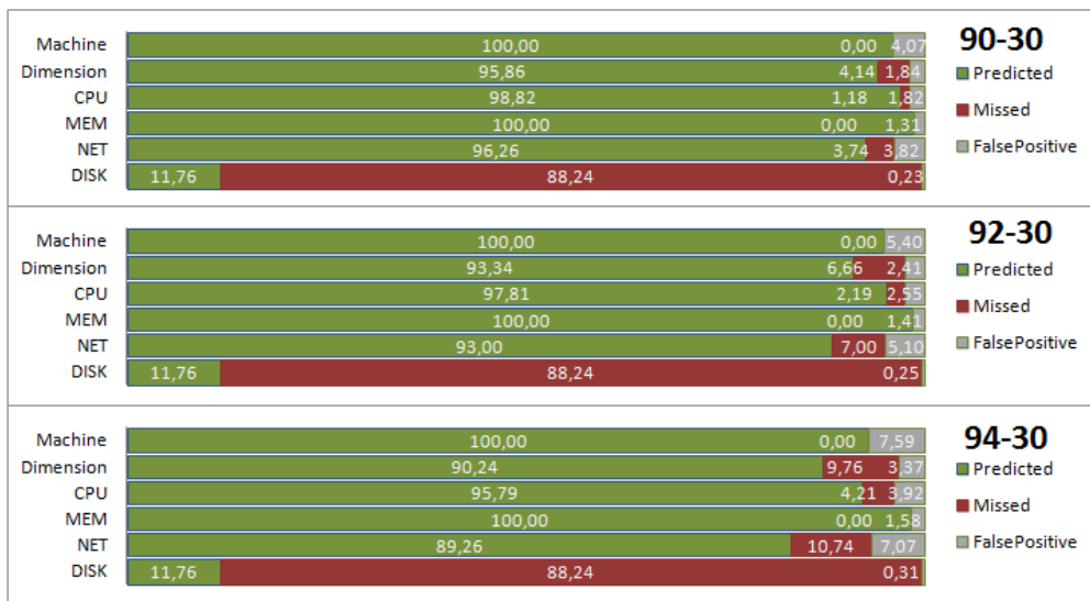
Figure C.5: NNAR (Neural Network Autoregression) with changing window size. The first number in the chart title is the confidence level, the second is the window size.
