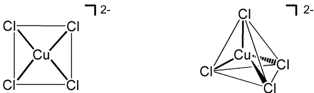
Figure 38 Schematically drawing of the square-planar (left) and tetrahedral configuration (right) of [\text{CuCl}_4]^{2-} .
