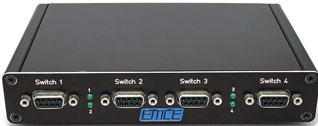
Figure 3.4: RF switch controller front view with 9-pol D-Sub connectors to the RF switches
