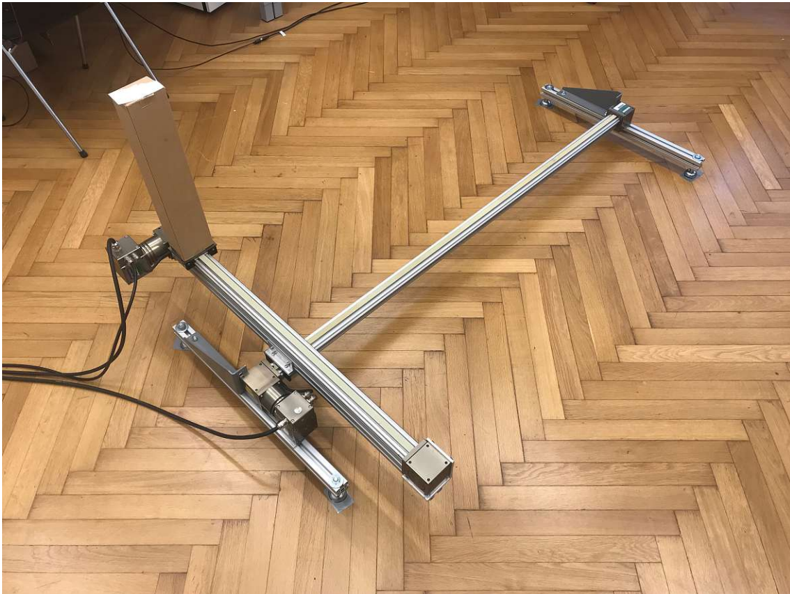
Figure 4.13: Tag positioner for precisely moving a tag during the measurements
