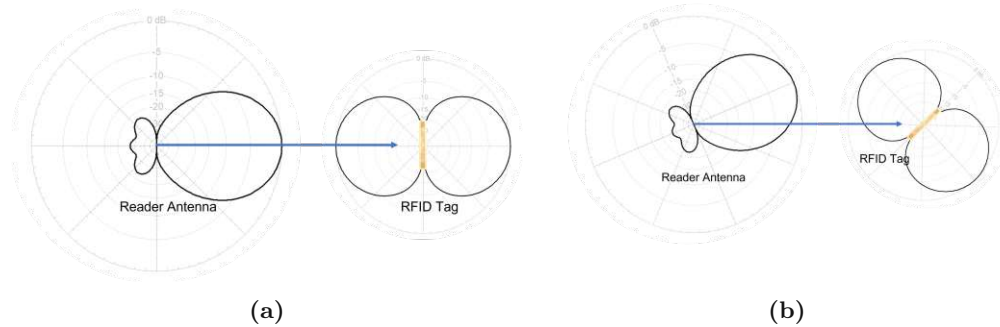
Figure 2.5: Scenarios for RSSI measurements; a) good, b) poor (for unknown antenna pattern)
