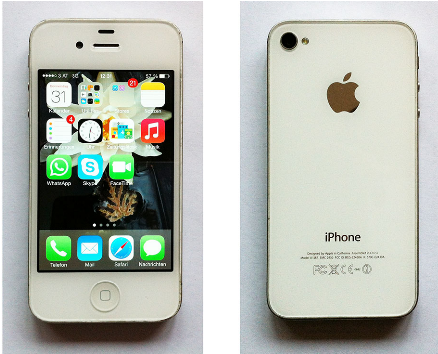
Figure 2.1: An Apple iPhone [47]: A current example of a smartphone, including a multi-touch screen, cameras in the front and the back as well as personalized applications and a custom background.
