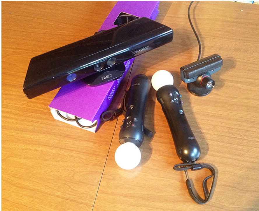
Figure 2.3: From left to right: A Microsoft Kinect Sensor, Sony PlayStation Move Controllers and the according PlayStation camera.
