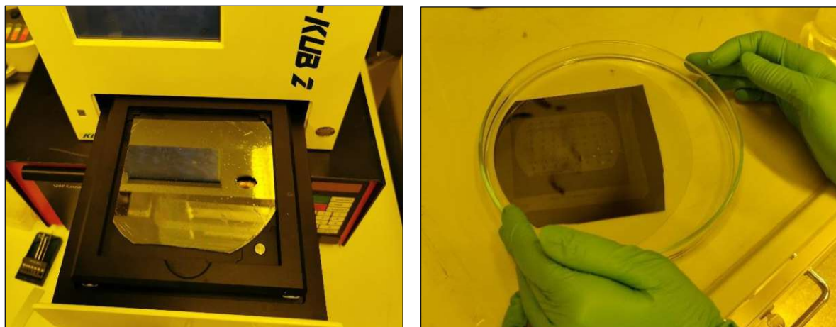
Fig. 117 left: Insertion of the appropriately cut wafers into the Kloé - UV-KUB 2 UV exposer; right: Development of the UV exposed wafers using the mr-Dev 600 SU-8 developer in a large glass petri dish – structures can be already distinguished after short treatment times.
