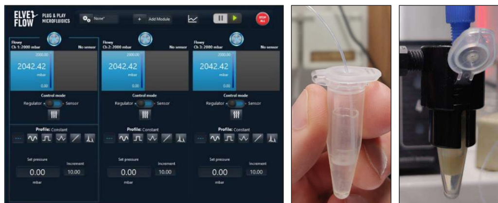
Fig. 124 - left: GUI of the Elveflow® microfluidic control software; middle: pre-drilled Eppendorf tube used to collect formed droplets during the encapsulation stage; right: Eppendorf tube containing the milky droplet layer on top of the transparent buffer oil phase.
