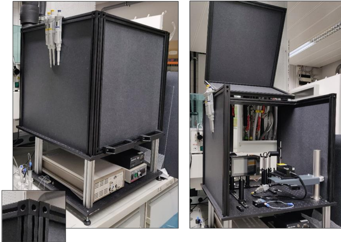
Fig. 107: Closed and opened from the whole set-up – back cover missing in open form due to easy accessibility during the construction process. All crucial instruments (high voltage amplifier, laser diode controller, PMT controller, ..) are mounted on an elevated stage below the covered optical assembly. Expansion: Close-up of the connectivity of the general cubical structure via RM15 construction cubes and XE25L structural rails
