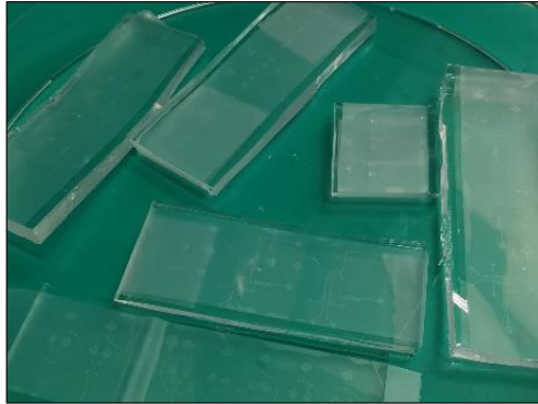
Fig. 89: Mass production of chips enabled by the manufacture of multiple master molds.
