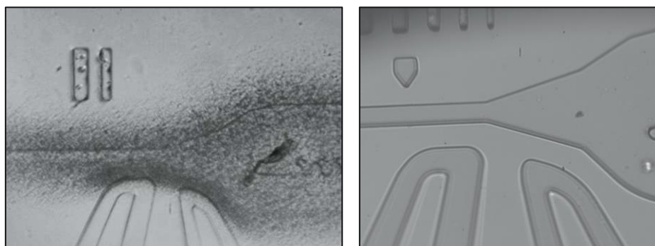
Fig. 88: Inexplicable darkening of the PDMS chips surrounding the microfluidic channels by prolonged treatment with 1 vol% tridecafluoro-1,1,2,2-tetrahydrooctyl)trichlorosilane solution ( left ). Limiting the reaction to maximum 5 minutes prevented this effect ( right ).
