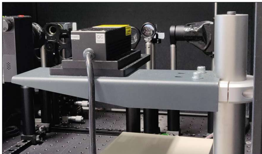
Fig. 106: Additional pedestal for flexible adjustment of the laser diode system – hinged clamps attached to the P250/M pole could be easily loosened to adjust the height of the assembly.
