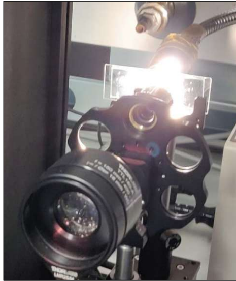
Fig. 109: Backlight illumination of the microfluidic chips with the flexible HL250-AS single fiber gooseneck microscope illuminator
