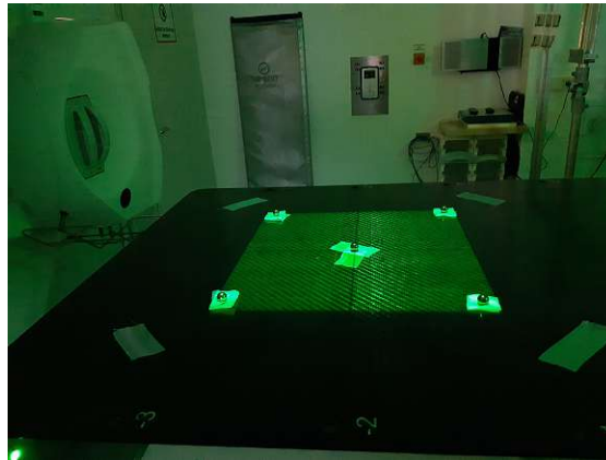
Figure 3.8: The Set-up of the measurements of the spheres. The spheres are situated at the four edges and at the centre of the detector.
