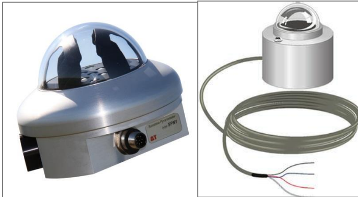
Figure 17: Sunshine pyranometer (left) for diffuse irradiance and pyranometer (right) for global irradiance measurement
