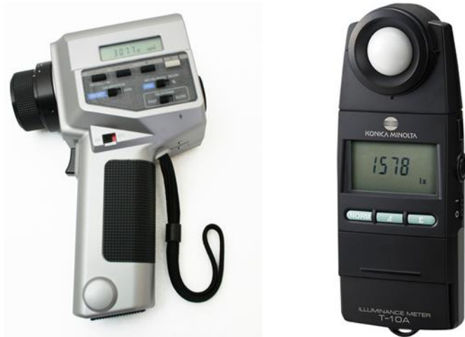
Figure 20: Luminance meter (left) and hand-held illuminance meter (right) used for reflectance measurement
