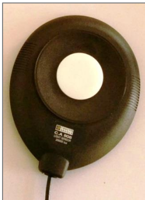
Figure 18: Indoor illuminance meter used in the experiment to measure work plane illuminance
