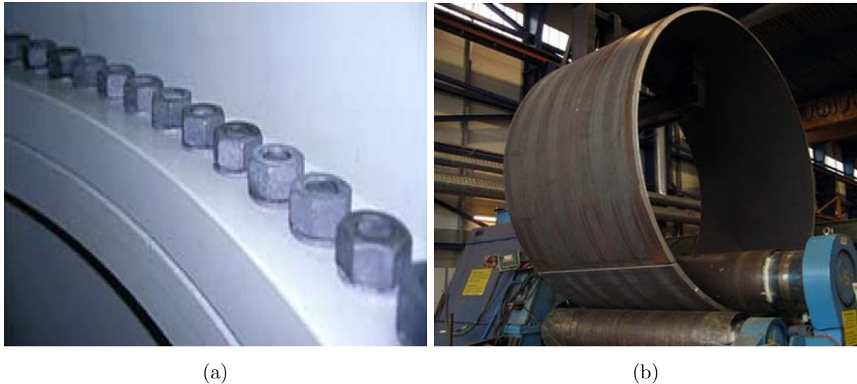
Figure 2.5: Steel tower; (a) bolt connection between segments, taken from [7]; and (b) rolled 40 mm thick steel sheet, taken from [8]
