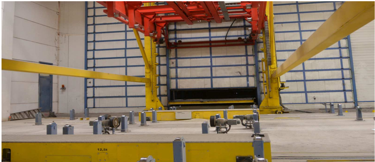
Figure 4.47: Storage and curing area of the double wall elements
