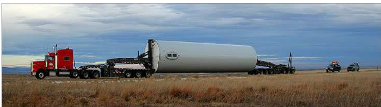
Figure 2.6: Transportation of a steel tower segment, taken from [9]
