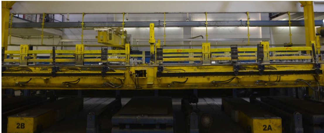
Figure 4.41: Lifting of the pallet with the first shells from the day before
