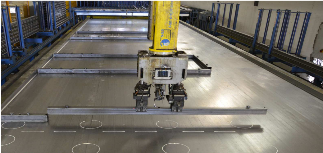
Figure 4.32: Forwork robot placing the lateral formwork profiles
