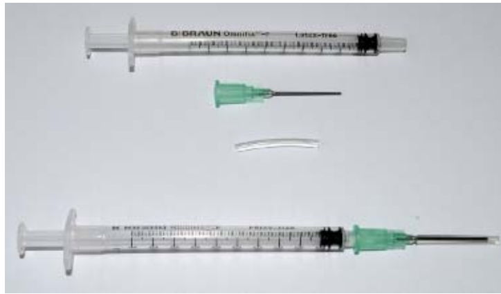
Figure 4.10.: A 1 mL syringe, a 0.8 mm cannula and a piece of rubber tube (top) that were combined (bottom) to create a tool for administering the particle solutions to the microfluidic channel.
