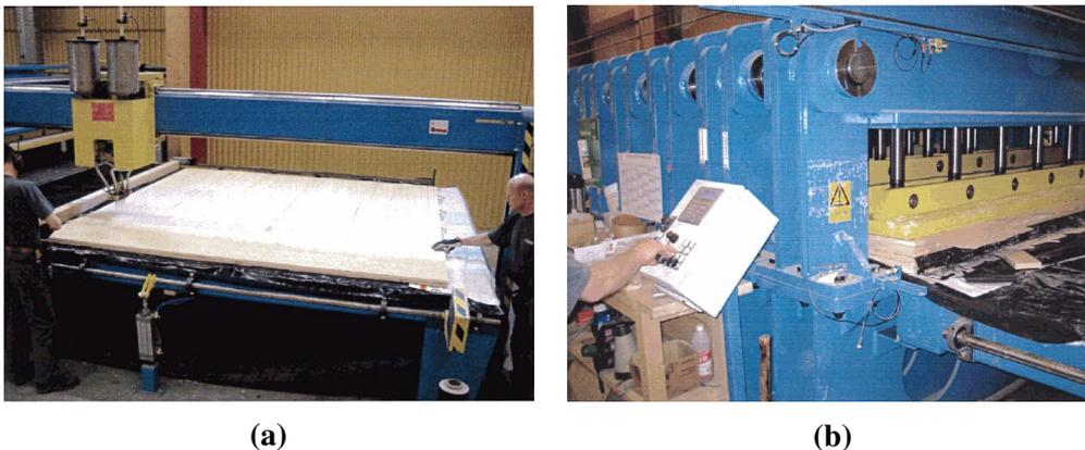
**Figure 4.2:** CLT production facilities at Setra factory in Dalarna, Midsweden. (a) Table for the manual setup of single layers and (b) pressing device for gluing
