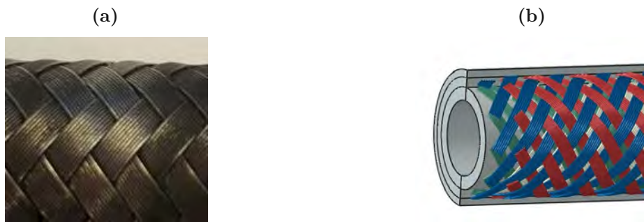
Fig. 4.1: Steel braiding embedded in the hydraulic hoses studied in this thesis; (a) photograph of an exemplary braiding structure, and (b) reconstruction of the overall structure of the hoses
