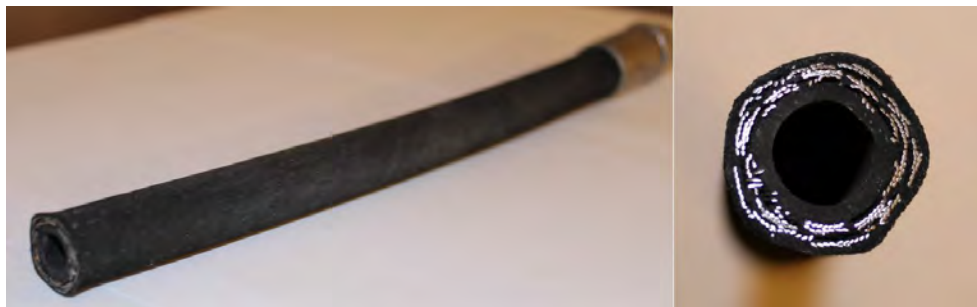
Fig. 2.1: Investigated material: steel-reinforced rubber hoses; photographs showing the investigated specimens (left) and one exemplary of the cross sections of the latter (right)
