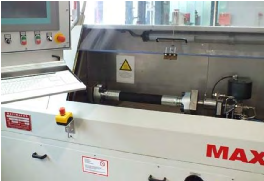
Fig. 1.2: Photograph of the device used for hydraulic testing of hoses [16]
