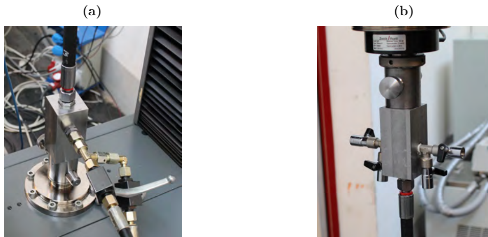
Fig. 3.4: Measurement setup: (a) connection on the machine base; (b) connection on the moving crossbeam
