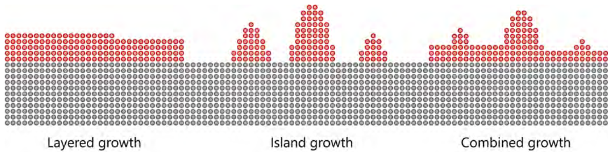
Fig. 2.5: Illustration of the three main growth modes observed during magnetron sputtering [35].
