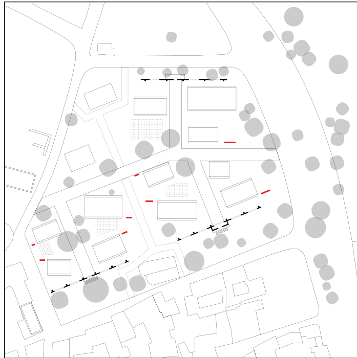
The wall extension, when possible, will add variation to each pavillion and it will support the privacy
