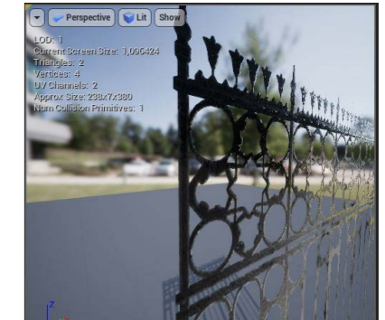
Abb. C-141: Gitter manuelles LOD 1 mittels Alpha-Map, 2 Triangles
