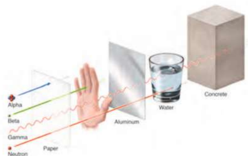
Figure 4 | Penetration levels of alpha, beta and gamma radiation types 6
