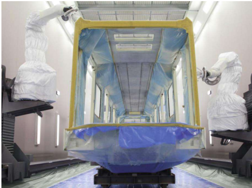
Figure 20: Fully automated painting process in the surface treatment facility.
