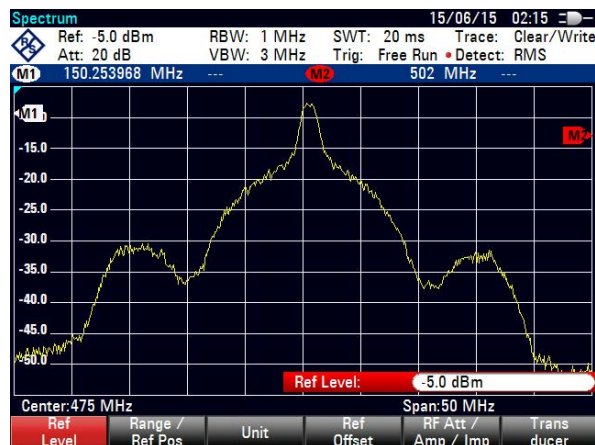
Figure 5.5: GPS L1 signal spectra observed in the Experiment 179a and visualized with a spectrum analyzer connected to an intermediate frequency (IF) channel in Hobart. The depicted IF spectra is down-converted from the RF domain using a local oscillator frequency of 1100 MHz.
