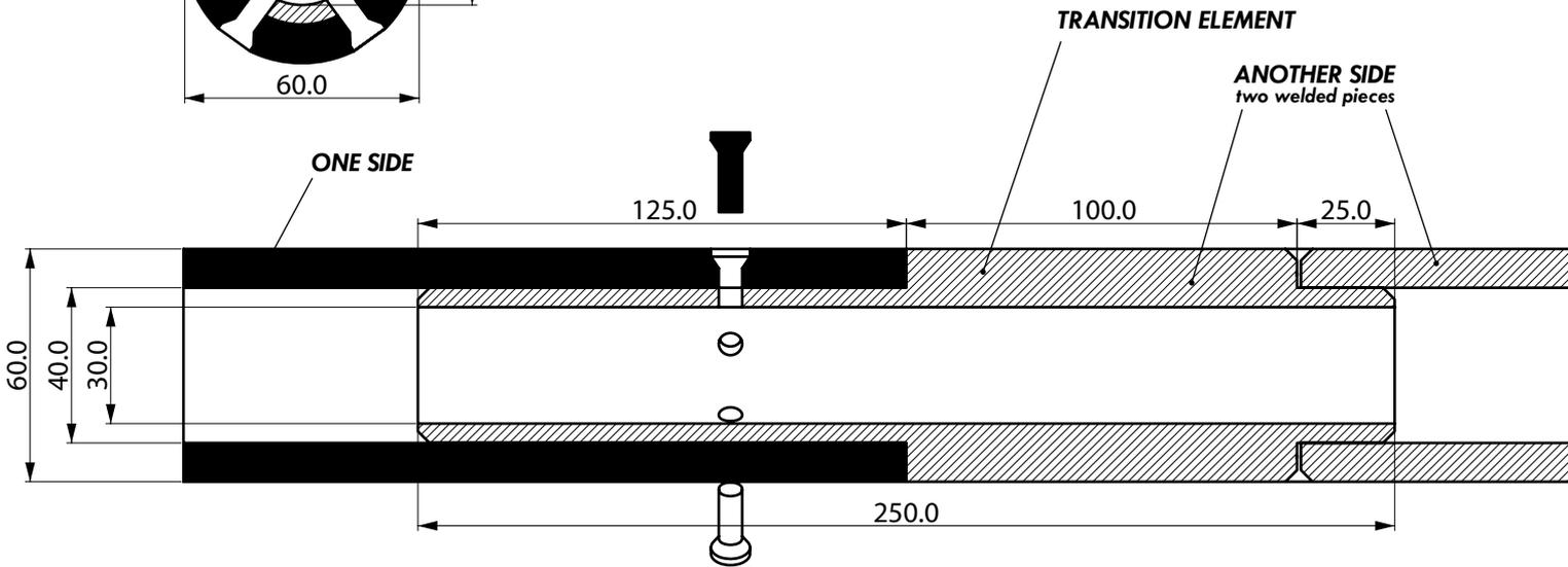
(for example *pemat* company) that can produce the elements already in right form and necessary length ( $l=2-2,5m$ ). By complex elements, all pipe parts will be welded together into one piece (drawing SP5).
