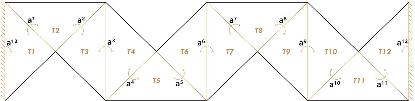
$a^n$  - degrees of freedom rotation along the triangle side axis (in each triangle of 2 of 3 of its ribs are involved)
