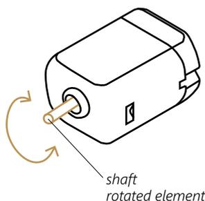
diagram SP12 "DC electric motor"
