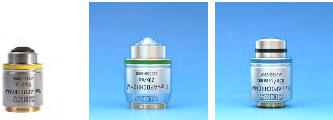
Figure 3.5: Objectives used in this thesis. 10x/0.3 [179] and 20x/0.8 [180] were used for structures larger than 200 \mu\text{m} . 63x/1.4 [181] was used for high resolution experiments.
