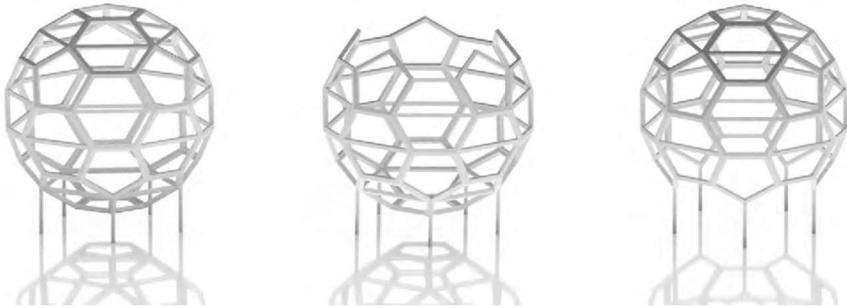
Figure 3.12: Buckyball design for Faraday wave experiments. Five rods fix the scaffold to the glass slide. Three designs - conventional buckballs (left), open top buckyballs (middle) and open bottom buckyballs (right) - were modeled to study the effect of geometry on the number of trapped cells. A central barrier for the base-hexagon element was added to reduce the pore-size.
