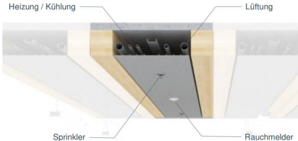
Abbildung 3.2: Deckenelement LCT-Life Cycle Tower, Dornbirn [18]
