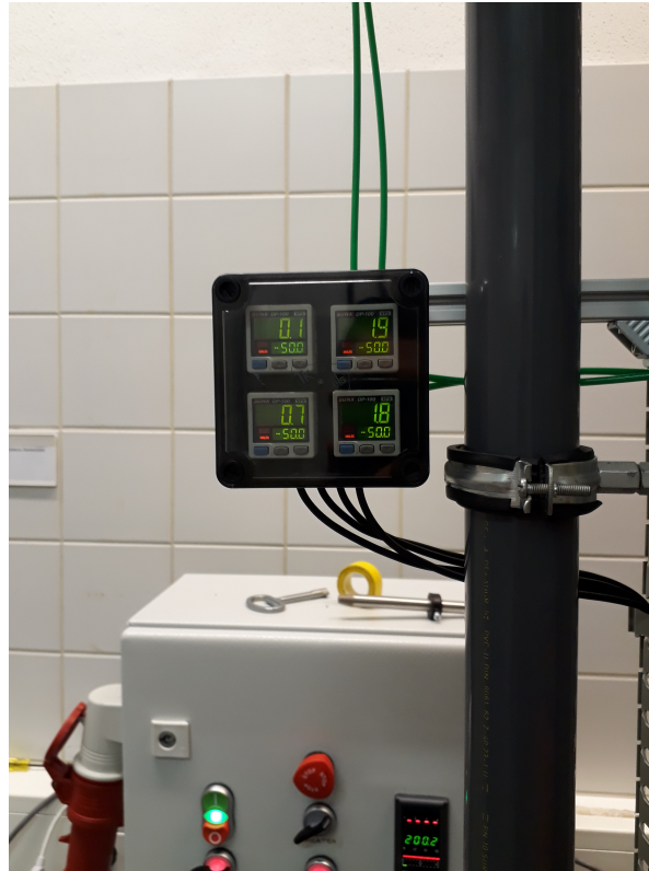
Figure 3.6.: Local pressure measurement of all four measuring points
