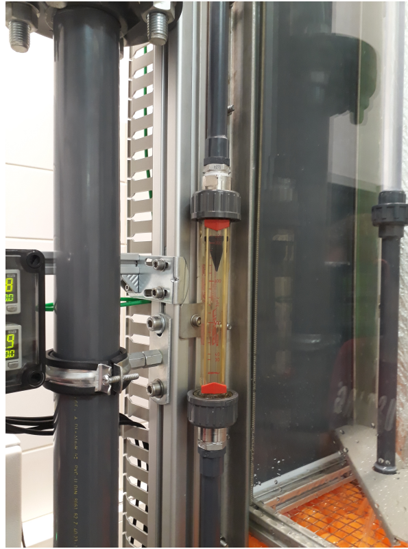
Figure 3.4.: Flowmeter for determining the water flow
