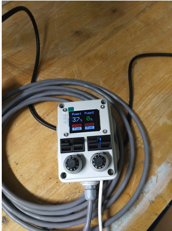
Figure 3.9.: Remote control unit for both pumps
