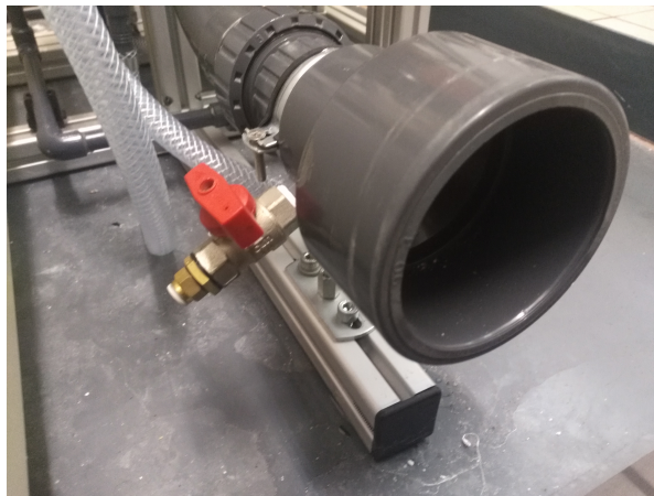
Figure 3.2.: Air- and additional gas inlet
