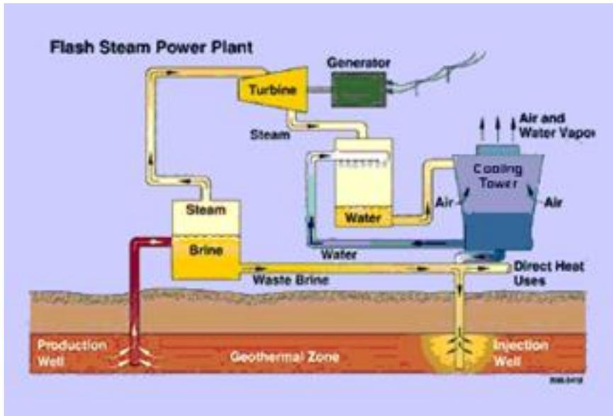
**Figure 26:** Flash Steam Power Plant System (from <http://geo-energy.org/basics.aspx>)
