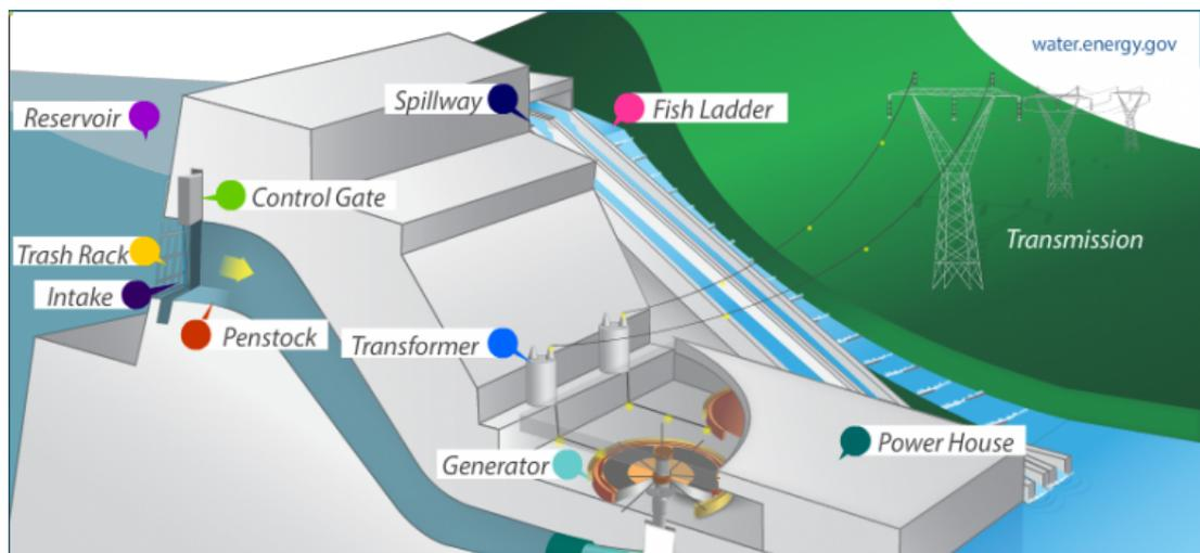
**Figure 30:** Hydroplant System Diagram (from <http://gubik.abidingtruthministry.co/hydropower-works/>)
