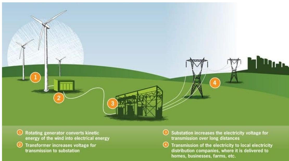
**Figure 8:** How wind turbines work (from <https://canwea.ca/wind-facts/why-wind-works/>)
