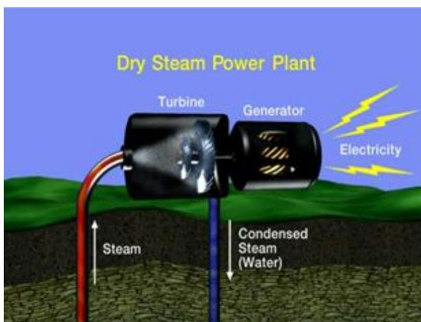
**Figure 27:** Dry Steam Power Plant Sys (from <http://geo-energy.org/basics.aspx>)
