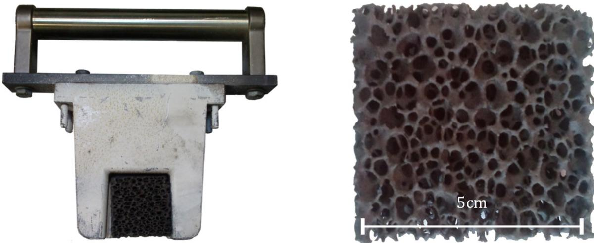
**Figure 23: Separator with filter (left), ceramic filter (right)**
