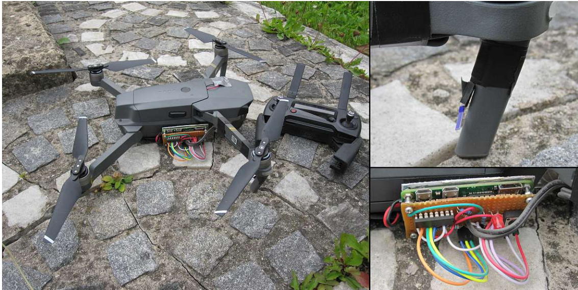
Figure 3.3.4: DJI MAVIC PRO with mounted temperature logger. For the RASPBERRY PI's power supply, the UAV's battery pins are used (red and black wire on top of the drone).
