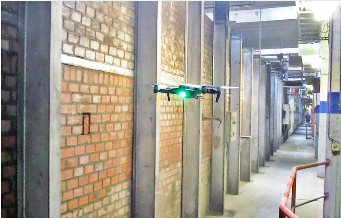
Figure 3.3.5: Area where the influence of temperature changes on the drone's flight behaviour was tested. On the left side, the side wall of a tunnel kiln can be seen (brick wall). Temperature increases in the course of the corridor from 20 °C up to 35 °C.
