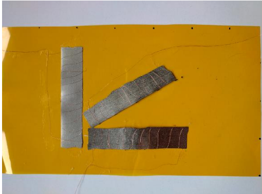
Figure 16 Sensor of “middle” width: three nanocrystalline ribbons of 10mm width and 50mm length.
