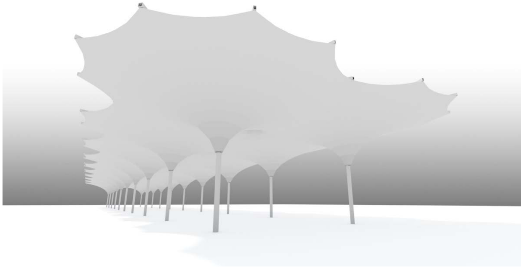
Figure 5.28 3D render of the suggested 100m module for use on the pedestrian walkways – Option 6: Cluster of 20 units.
