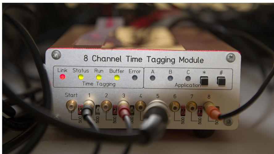
**Figure 25:** Time tagging unit from Roithner Laser Technik, TTM8000. Channel 1 and 3 were assigned to detectors 0 and 1, channel 5 was assigned to the GPS pulse-per-second signal and channel 8 was assigned to the RS-232 port of the Alice PC.
