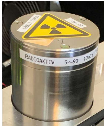
Figure 6.8: ^{90}\text{Sr} source with 10 mCi / 370 MBq used for open shutter measurements.
