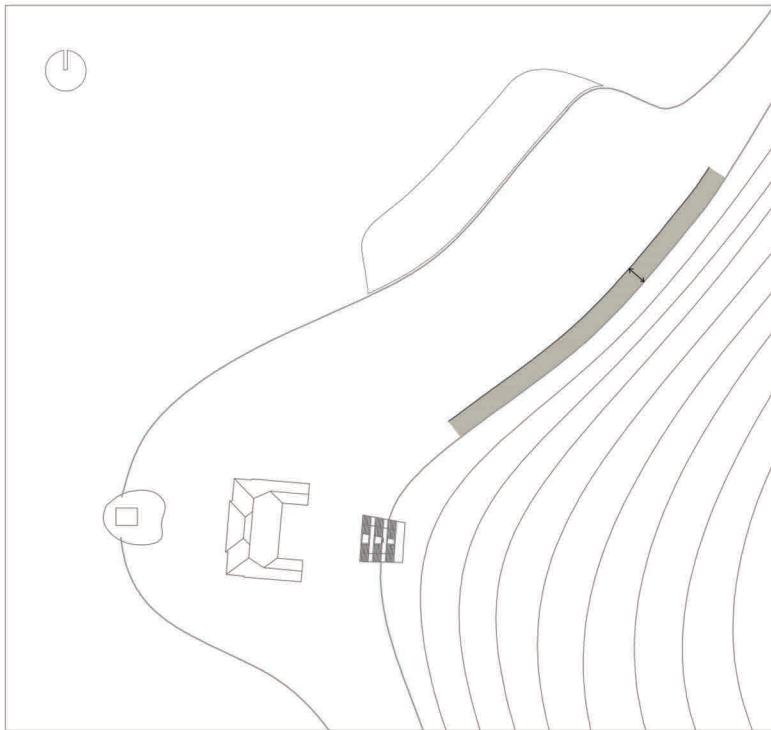
7 meter distance between the Health center and the hill (for more sunlight)
