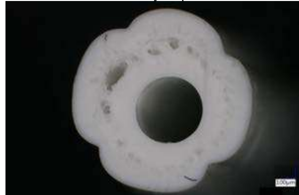
Figure 1: Micro-structured PES-PVP hollow fiber membrane spun with a self-developed spinning plant.
