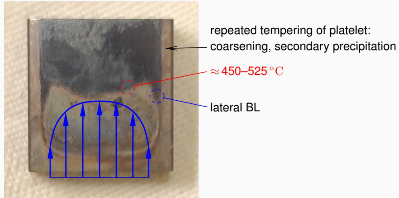
PM X190CrVMo20-4-1, Ultramid® A3W (PA66, no fibres), 210 blasts ( $300\text{ cm}^3/\text{s}$ )
