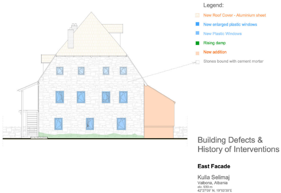
Fig. 200 Building defects and history of interventions in the East façade of the building
