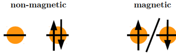
Figure 2.2: Isolated interacting impurity with a single non-degenerate orbital (orange), which can be at most doubly occupied. The energetically degenerate magnetic states are formed by the singly occupied impurity site with spin \sigma = \uparrow, \downarrow .
