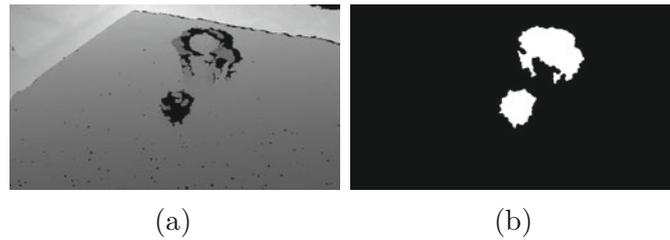
Figure 3.6: Depth image of a scene with transparent objects (a) and resulting mask after processing the invalid depth values (b).
