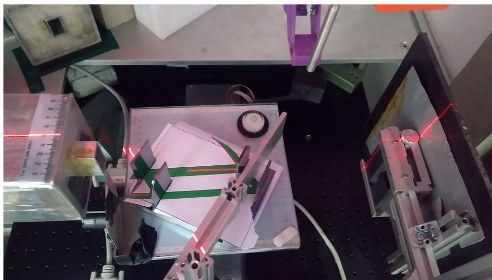
FIG. 3.4 – Close-up of the skew-symmetric interferometer with phase shifter, aperture (right) and collimators (left). Neutrons move from right to left.
