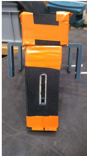
FIG. 3.7 – Front view of the shielding of a pencil detector mount (empty).
