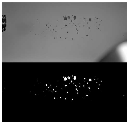
(c) Pellet #234, 100% Ne, 25° shatter tube, 202 m/s pellet speed.
