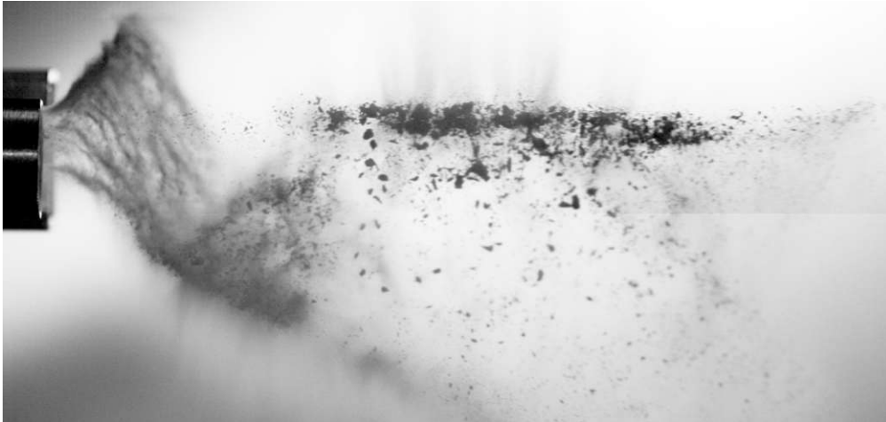
Figure 4.15. Frame showing a pronounced spiral dust patten produced by pellet #1098 (8 mm diameter) in a circular 25° shatter tube.
