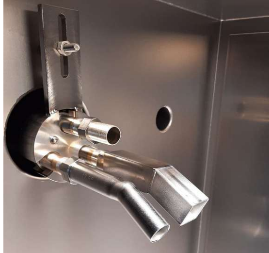
Figure 3.5. Photograph of the shatter heads in the shattering test chamber. At the topmost barrel, no shatter tube is mounted. 12.5° mitre-bend shatter tubes with a circular (left) and rectangular (right) cross-section are screwed onto the bottom left/right barrels.
