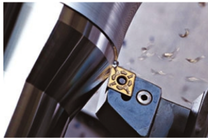
Figure 1.2.1: Tool machine working under dry conditions [22].
