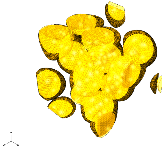
Figure 4.1.4: Deformed (solid mesh) and undeformed (shaded solid) TiN particles after transformation, as obtained for one unit cell of type UCSP for an Al mole fraction x = 0.50 , \xi^{(\text{TiN})} = 0.2 and unconstrained conditions. The deformation scale factor is 21.576.
