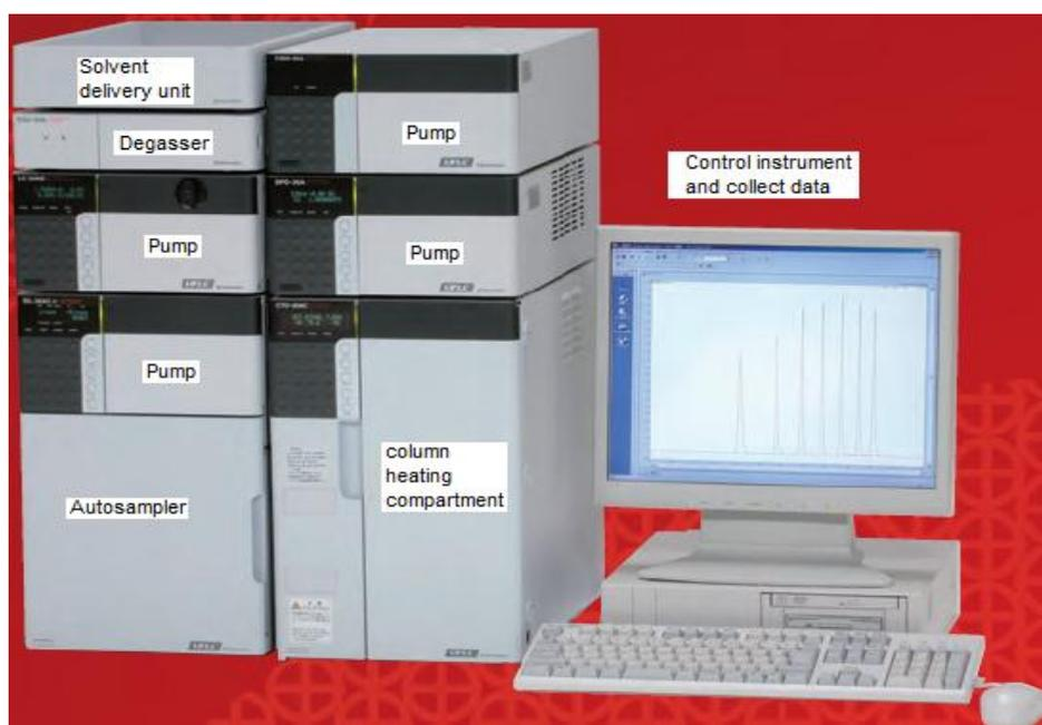
Figure 6: Simadzu HPLC instrument [66]
