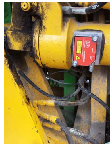
(c) Tamping arm with applied laser range finder
