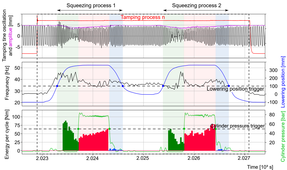
(b) Calculated data showing tine oscillation, amplitude (raw and smooth), frequency, energy per cycle and the triggers for tamping process subdivision
