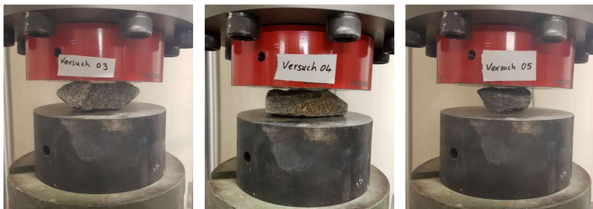
Figure 7.25: Single grain compression test on three grains of fine-grained granite
