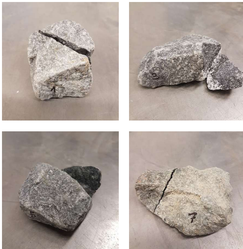
Figure 7.26: Effect of particle size ( d is defined as the distance between two plates at failure) on single particle tensile strength
