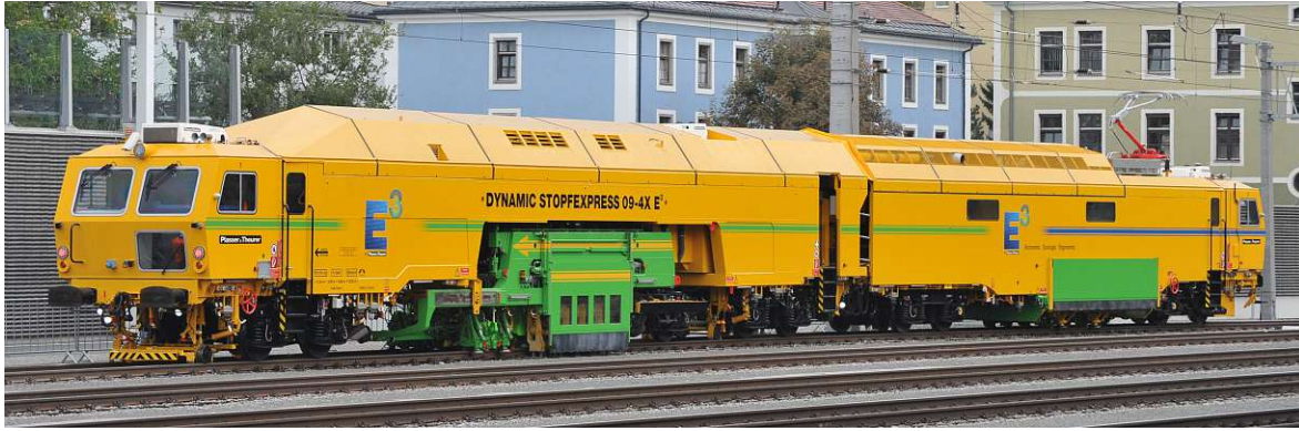
Figure 5.1: Tamping machine Dynamic Tamping Express 09-4X E 3 (©Plasser & Theurer)
