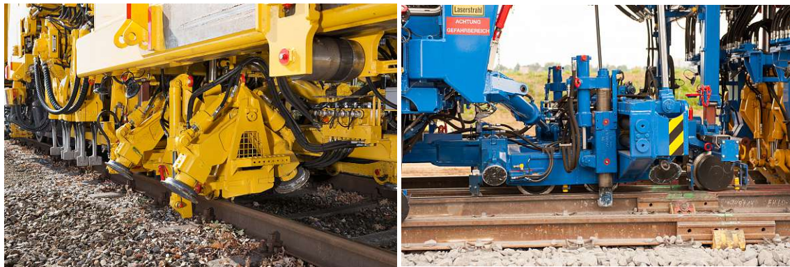
(a) Roll lifting clamps and double-flange lining of a plane tamping machine (b) Roller lifting clamps with lifting hooks and lining rollers for universal use in turnouts
