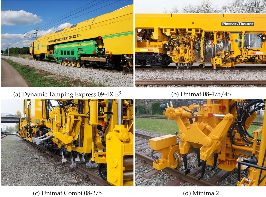
Figure 4.11: Tamping machines (©Plasser &amp; Theurer)
