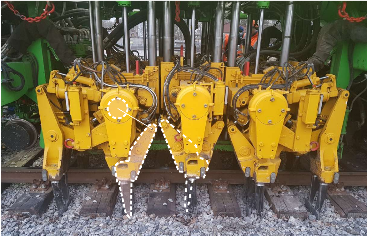
(a) Tamping unit of the Dynamic Tamping Express 09-4X E 3 with one highlighted tamping arm
