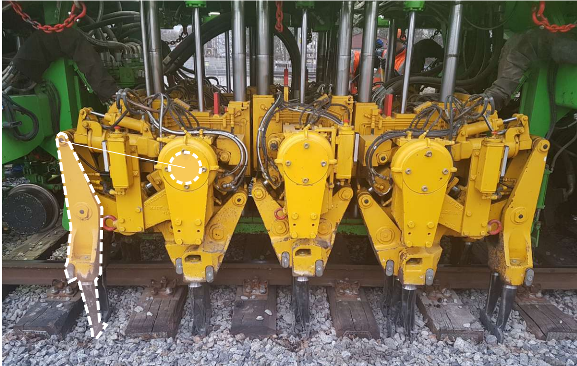
(a) Tamping unit with highlighted tamping tine N° 64
