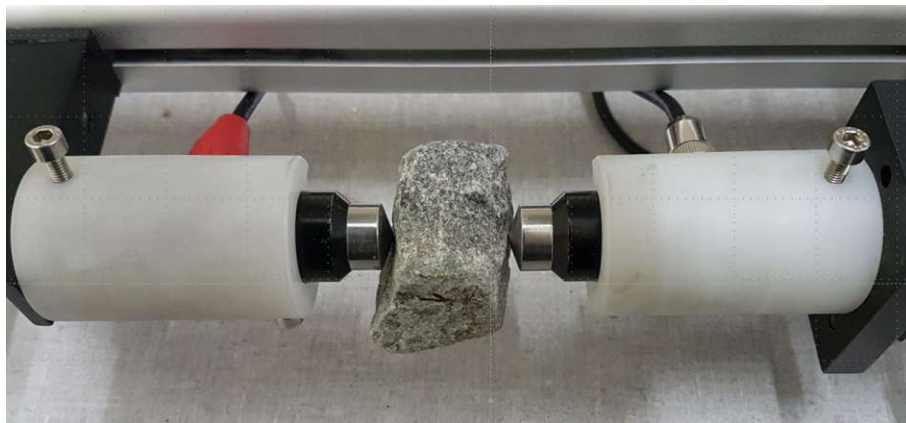
Figure 2.17: Ultrasonic Pulse Velocity test on a single ballast grain
