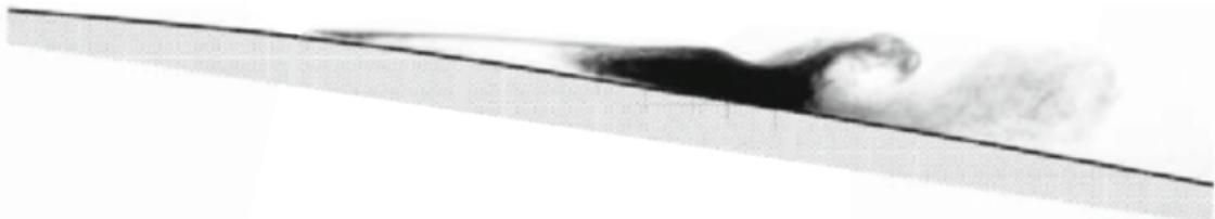
Smoke flow visualisation of a LSB on an Eppler 387 airfoil at  $\alpha = 2^\circ$  and  $Re \approx 10^5$  [G. Cole, T. Mueller, 1990]
