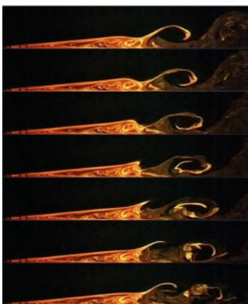
LSB in a laminar water tunnel: A-vortex generation cycle at  $Re \approx 10^5$
