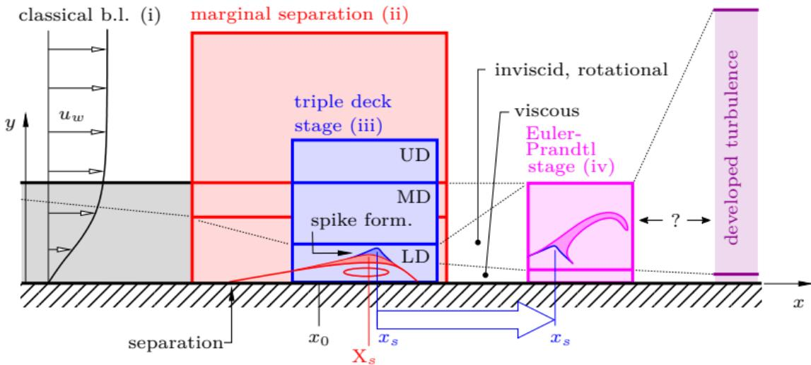
Early stages of the laminar-turbulent transition process
