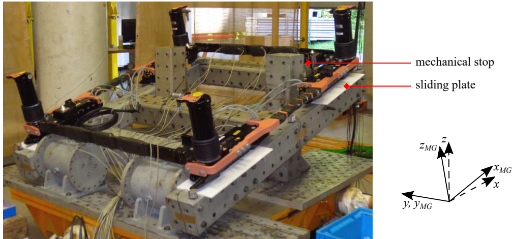
Figure 2.14: Vibration test of the magnetic track brake
